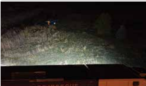
PERIMETER LIGHTS 1 WHELEN 900 SERIES AND 2 WHELEN M9S ON EACH SIDE OF THE TRUCK
