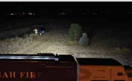
PERIMETER LIGHTS 1 WHELEN M9 AND 2 FIRETECH FT-B-45 (46" LED STICKS) ON EACH SIDE OF THE TRUCK
